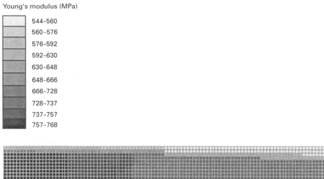
Figure 8 Model of the inhomogeneous paper structure used in the simulations.
