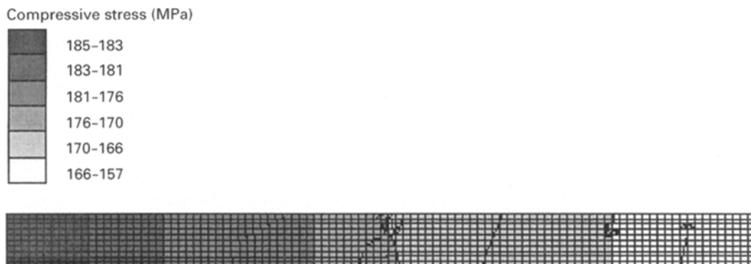
Figure 9 Calculated stresses in the thickness direction in an inhomogeneous paper structure. The paper model was compressed 30%.
